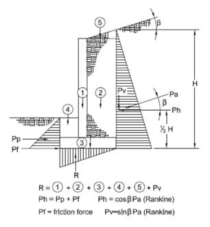
Figure 2.1 Free-body of cantilevered retaining wall
