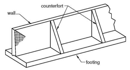
Figure 1.1 Counterfort retaining wall
