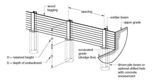
Figure 21.1 Typical soldier beam construction
