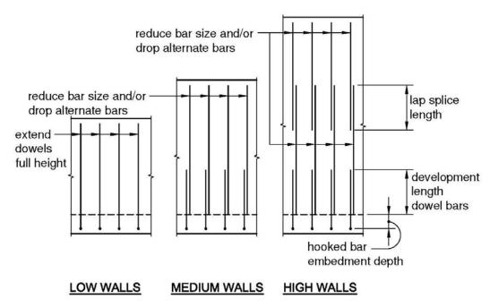
Figure 7.1. Reinforcing placement in stem
