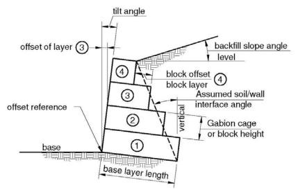
*Figure 15.1* Example of gabion wall analysis section Lateral pressures are computed by the Coulomb equation shown in Figure 15.2.
