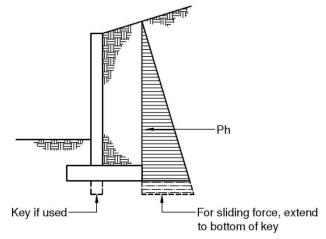
Figure 8.1 Overturning moments for a cantilevered retaining wall
