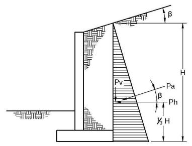
Figure 8.3 Vertical Component of Active Pressure
