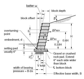
Figure 16.2 Forces on gravity SRW walls
