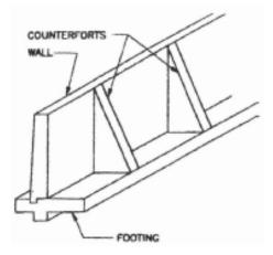
Figure 11.1 Typical counterfort wall
