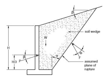
Figure 5.3 Rankine free-body of lateral forces on stem
