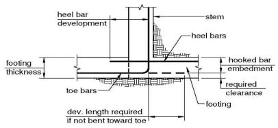
Figure 9.1 Hooked Bar Bend Requirements
