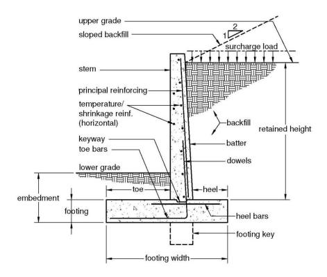
*Figure 1.2* Retaining wall terminology
