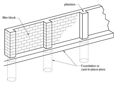
Figure 18.1 Pilaster masonry wall
